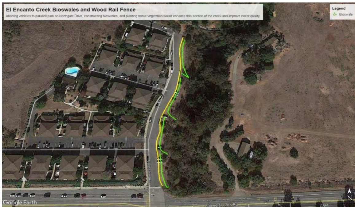
Figure 54. A wood rail fence (yellow line) along the east side of Northgate Drive would prevent vehicles from parking in dry weeds within the El Encanto Creek SPA, reducing fire hazards, improving water quality, improving habitat conditions, and enabling planting of native riparian species. Bioswales (green lines) would convey runoff and filter stormwater pollution from the street runoff before it enters the Creek. Google Earth. 2019.
