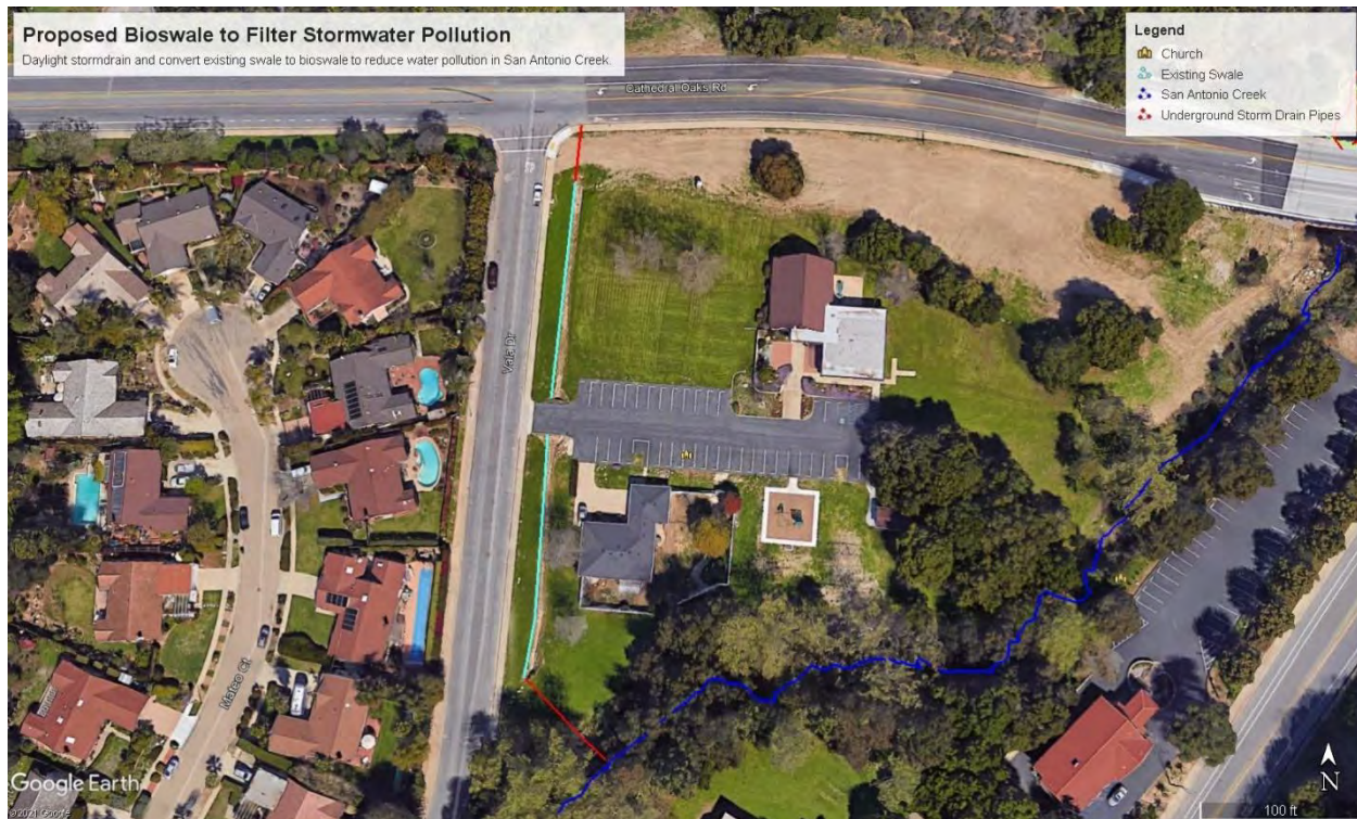
Figure 303. The red line depicts the storm drainpipes, and the light blue line is the existing 390 foot-along swale paralleling Vala Drive. The southern storm drainpipe should be daylighted, and, along with the existing swale should be converted into a bioswale and planted with high uptake native vegetation to filter pollutants from stormwater runoff before discharging into San Antonio Creek. Google Earth. 2019.
