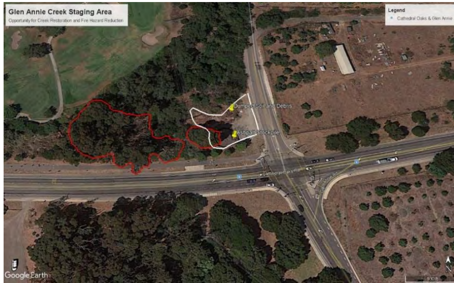
Figure 92. A staging area for road projects (white polygon) at the Cathedral Oaks Road and Glen Annie Road intersection includes an improperly contained and uncovered asphalt stockpile (black polygon), eucalyptus trees (red polygons), other invasive plants, and dumped dirt and debris. Google Earth. 2019.
