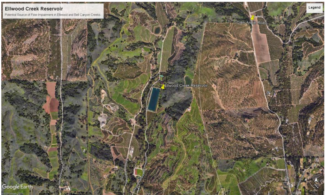
Figure 45. The Ellwood Creek Reservoir covers roughly five acres adjacent to the Creek and is likely supplied with water from the Creek or from shallow wells located in the vicinity of the Creek. It may therefore contribute to flow impairments in the Creek. Google Earth. 2019.
