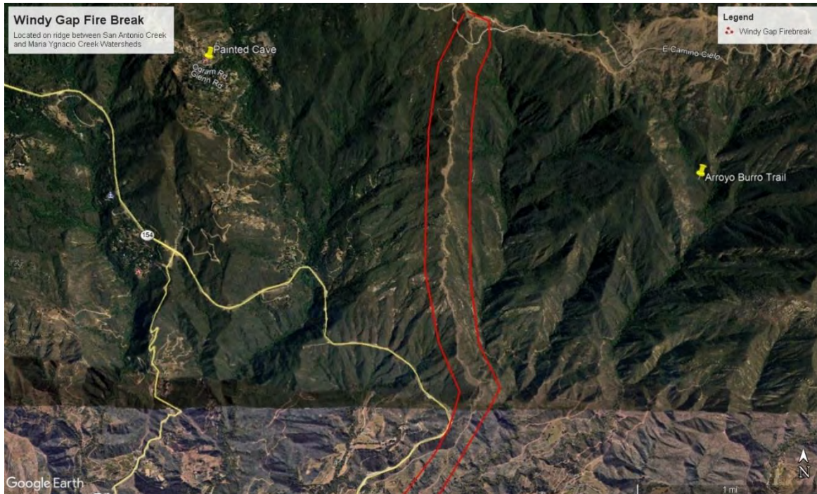
Figure 286. The Windy Gap Firebreak located between the west fork of San Antonio Creek and Maria Ygnacio Creek should be seeded with native grasses and fire-resistant native vegetation to mitigate erosion.
