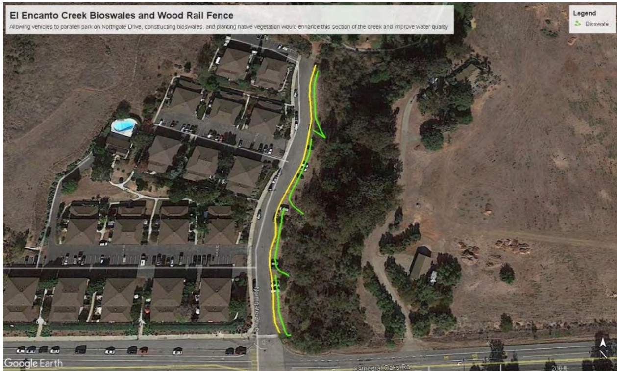
Figure 54. A wood rail fence (yellow line) along the east side of Northgate Drive would prevent vehicles from parking in dry weeds within the El Encanto Creek SPA, reducing fire hazards, improving water quality, improving habitat conditions, and enabling planting of native riparian species. Bioswales (green lines) would convey runoff and filter stormwater pollution from the street runoff before it enters the Creek. Google Earth. 2019.
