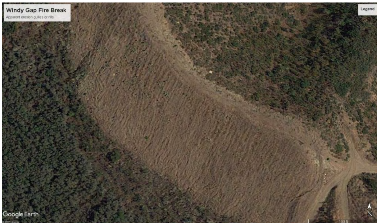
Figure 288. Erosion gullies or rills were present on the Windy Gap Firebreak in 2019 despite the installation of erosion control water bars. Google Earth. 2019.
